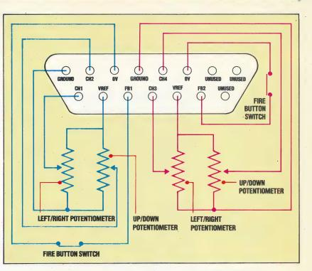
can be obtained. Turning the volume control on a radio or record player is essentially moving the middle connection across the resistance of the volume control potentiometer. In an analogue joystick the movement of the middle connection is made by moving the joystick handle.
